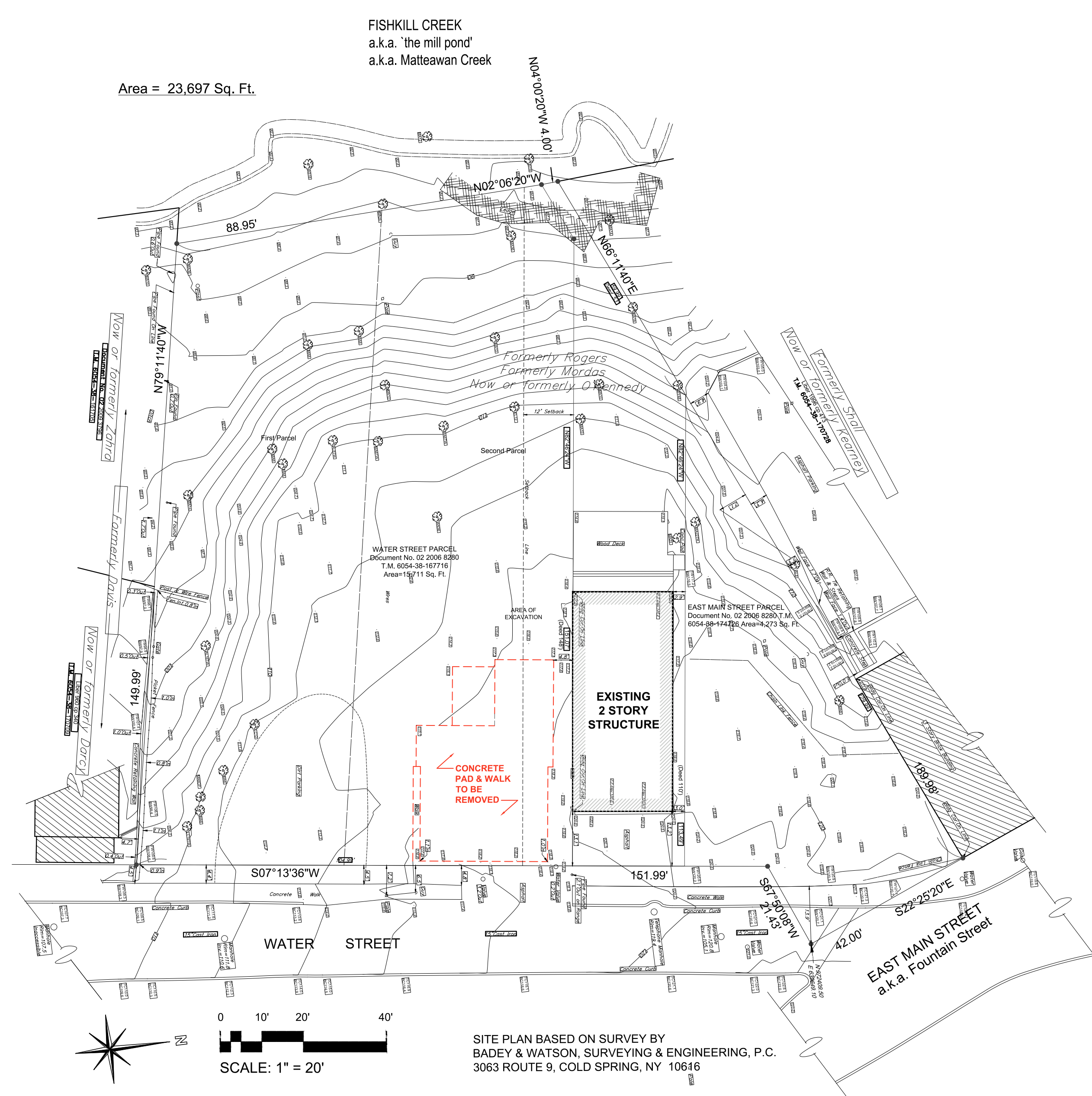
Site Demolition Plan Scale: 1" = 20'
