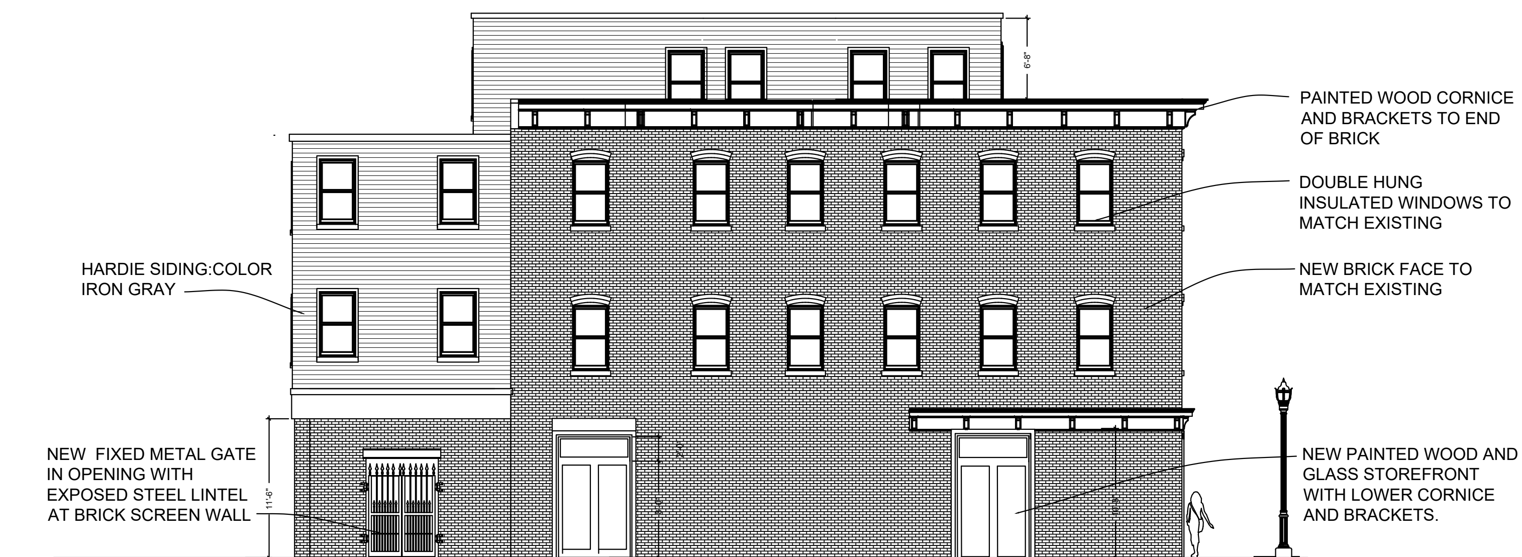
Side Elevation (Digger Phelps Court) Scale: 1/2" = 1'-0"
