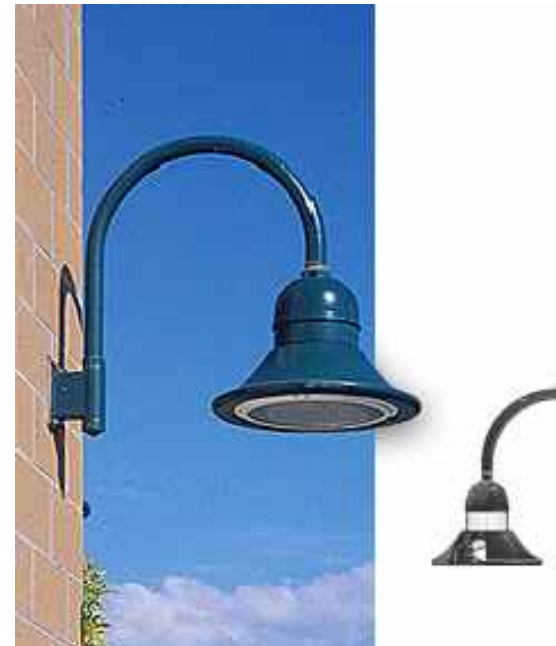
WALL MOUNTED LIGHT (L2) SELUX LIGHTING "BETA PENDANT" WALL MOUNTED FIXTURE, MODEL #BPC-L-R2-1-H50-BK-120-HS-PC WITH LOW GLARE CUTOFF SHIELD, COLOR: BLACK, PHOTOCELL CONTROL, OR APPROVED EQUAL. MOUNTING HEIGHT = 12 FEET
