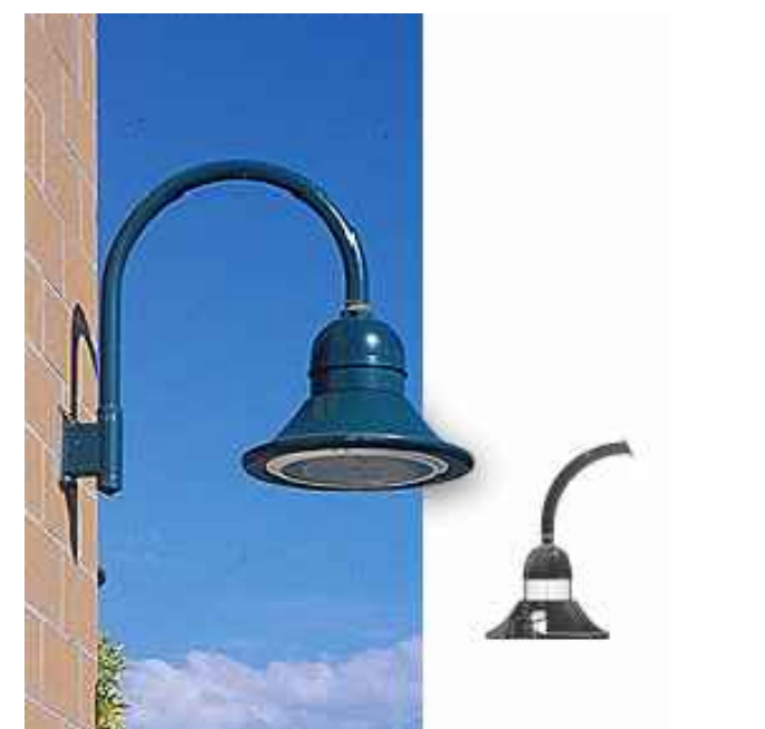
WALL MOUNTED LIGHT (L2) SELUX LIGHTING "BETA PENDANT" WALL MOUNTED FIXTURE. MODEL #BPC-LR2-1-H50-BK-120-HS-PC WITH LOW GLARE CUTOFF SHIELD. COLOR: BLACK. PHOTOCELL CONTROL. OR APPROVED EQUAL. MOUNTING HEIGHT = 12 FEET
