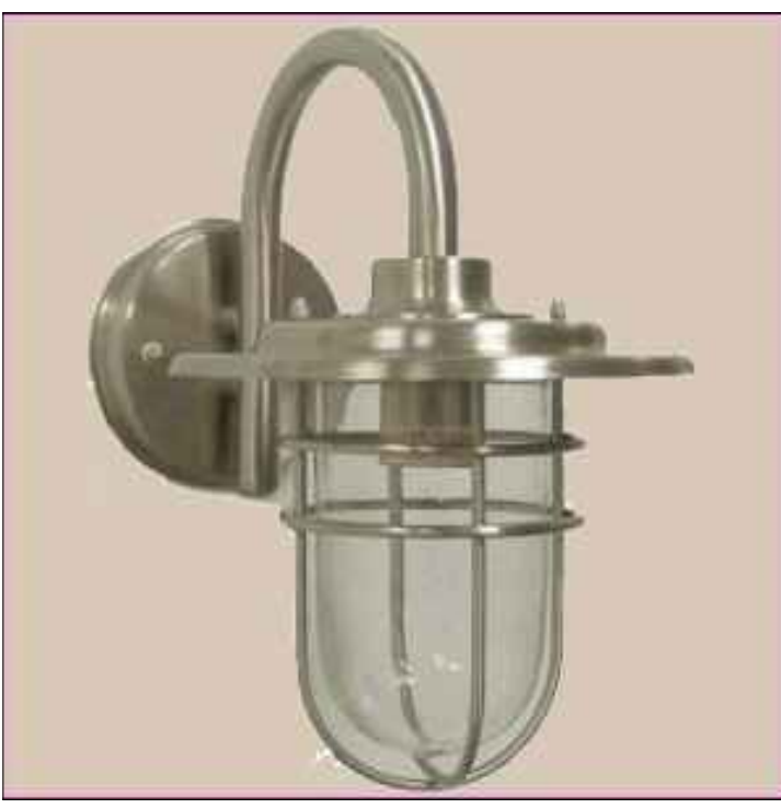
WALL MOUNTED HOUSE LIGHT (L1) ARK LIGHTING - WALL MOUNTED FIXTURE, MODEL #AW1002, 100W, COLOR: STAINLESS STEEL, FROSTED GLASS GLOBE OPTION, OR APPROVED EQUAL. MOUNTING HEIGHT = 8 FEET
